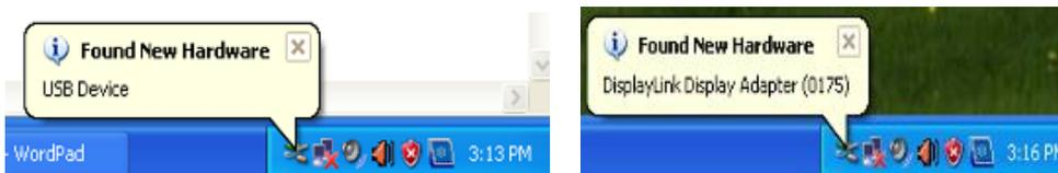
When setup is finished, a monitor icon is created in the system tray at the bottom of the monitor screen, and the information for the installed USB monitor is displayed.
